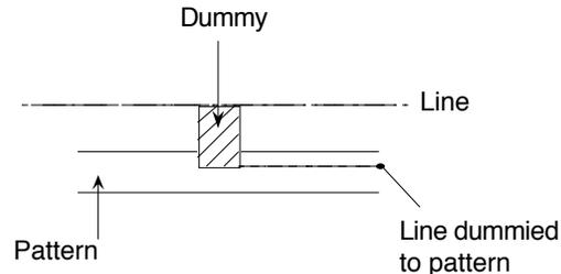
25.1.12 Using a dummy stick, transfer the shape of the centreline back on to the pattern (but a dummy's width in). Make a mark about every 100mm. Do the same with the chine line.
